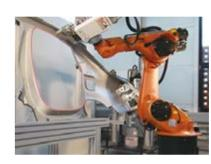
DuPont™ BETAMATE™ structural adhesives used to bond body structures
