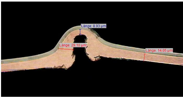
Poor copper throwing power
