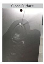
Picture 5: Water-break-free test. Insufficiently cleaned surface (left), well-cleaned surface with water film (right).
