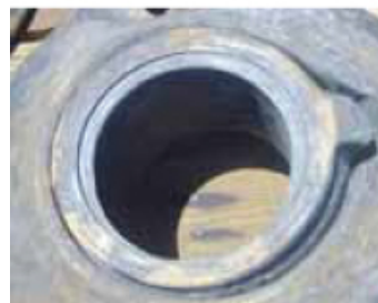
Metal impregnated graphite 3.5 year service 0.5" (12.7mm) Wear, shaft damage Not serviceable
