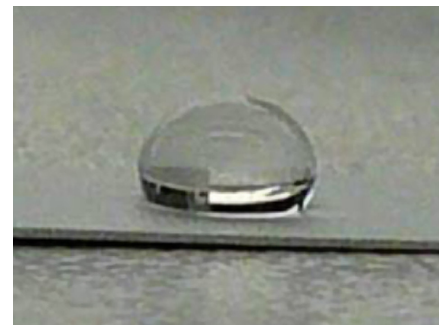
With SOLDERGUARD™ 100 Treatment After 1 hour @ 155°C
