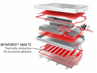
BETAFORCE<sup>™</sup> 2800 TC exhibits appropriate elongation to manage the potential temperature difference between the cooling unit and the cooling plate. Note - not an illustration of e-tron battery system.
