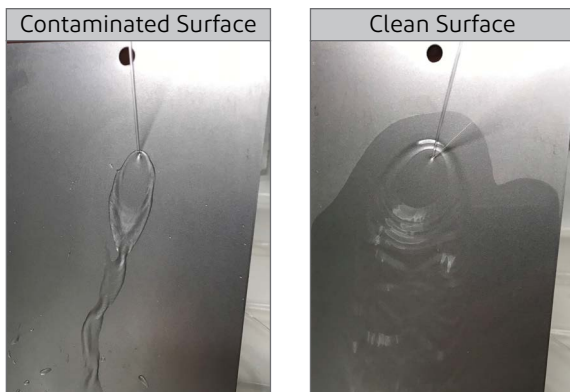
Picture 1: Water-break-free test. Insufficiently cleaned surface (left), well cleaned surface with water film (right).
