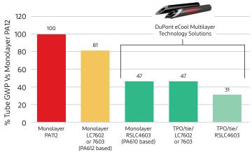
Values based on DuPont LCA estimations using cradle-to-gate material contributions to the tube assembly's GWP. Actual values may vary based on specific grade, tube material content, and tube dimensions. (Source: DuPont)
