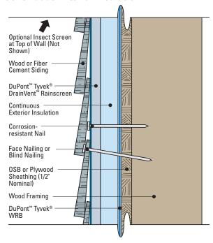
Install continuous exterior insulation according to manufacturer's recommendations. Install DuPont™ Tyvek® DrainVent™ Rainscreen over continuous exterior insulation, then install wood siding or cement cladding over DuPont™ Tyvek® DrainVent™ Rainscreen according to the cladding manufacturer's recommendations.
