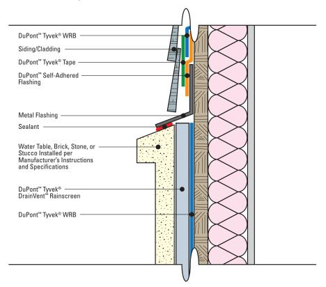
Option 2: DuPont™ Tyvek® DrainVent™ Rainscreen Installed Behind Siding/Cladding and Lower Facade
