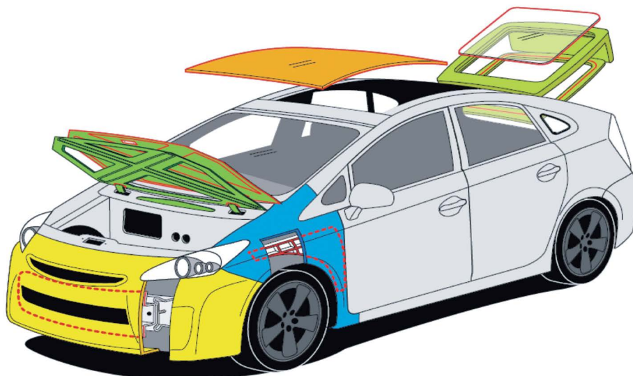
Figure 2 - Potential application areas of bonded hybrid composites.
