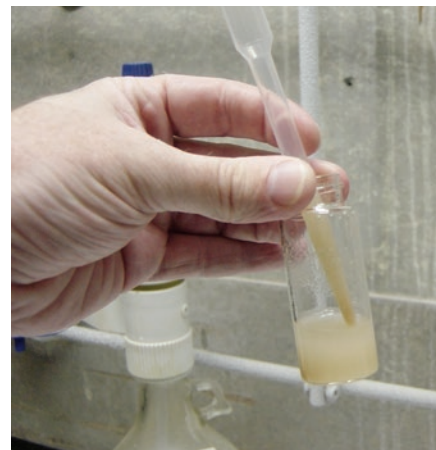
Figure 6 – Sample Resin Suspension
