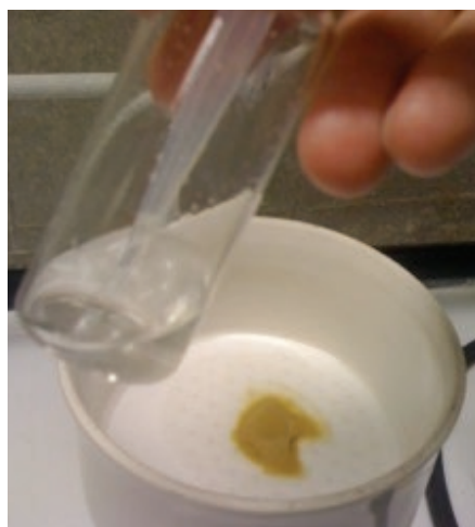
Figure 9 – Rinsing Vial and Wet Cake
