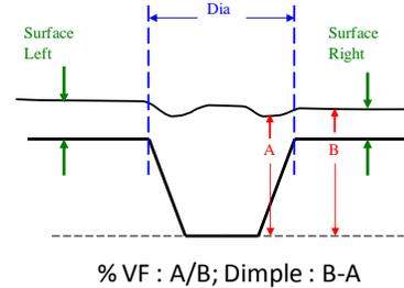
FIGURE 2. Dimple and void measurements
