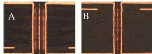
FIGURE 3. Through hole throwing power >80% for (A) 0.15mm and (B) 0.25mm diameter through holes.
