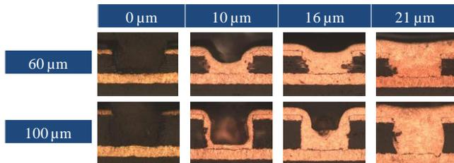
FIGURE 1. Plating performance as a function of surface copper thickness for 125 μm diameter vias
