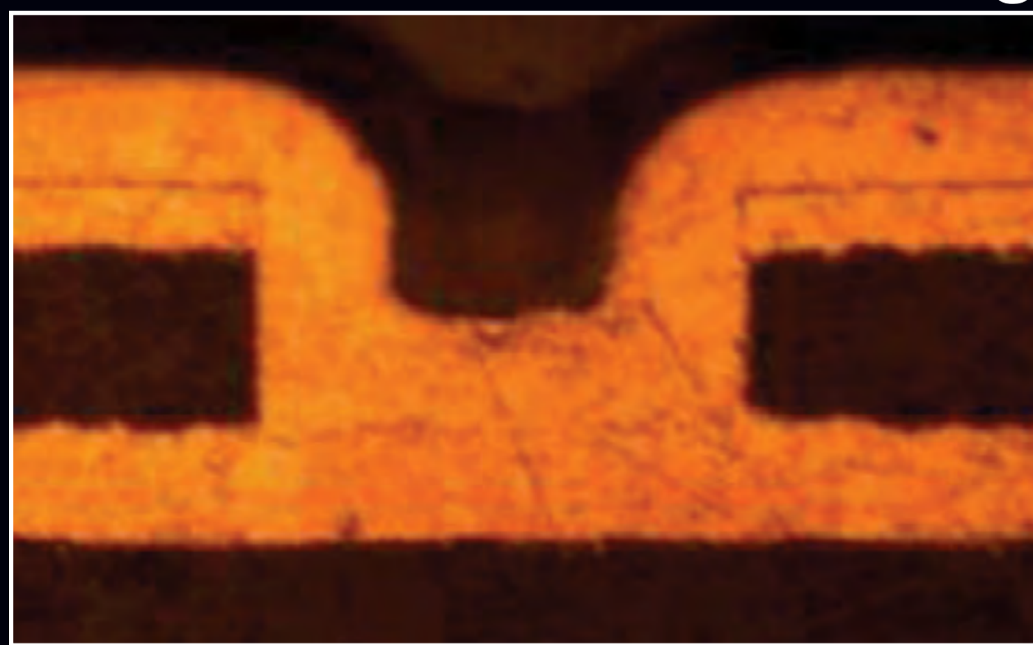
Figure 1: Microvia conformal plating • 100 μm φ x 60 μm BMV-Eless • Throwing Power = 91%
