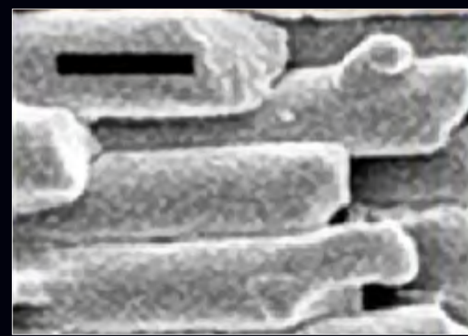
Excellent glass fiber coverage and ultra fine grain structure 优异的玻纤覆盖能力及细致的化铜沉积
