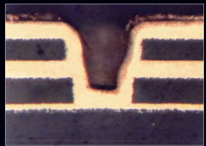
Excellent coverage in microvia 深盲孔优异的镀层覆盖能力
