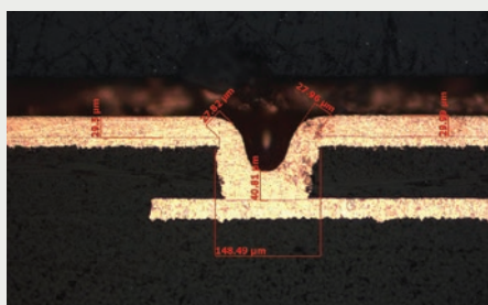
Figure 1: Microvia conformal plating • 150 μm φ x 100 μm BMV-Eless • Throwing Power = 135%
