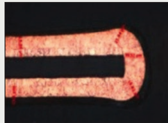
For SinYang 0.330Z ED Copper Foil, PI Thickness: 1 mil Throwing Power= 207% Knee Throwing Power= 147%
