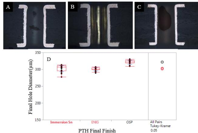
FIGURE 9 VERTICAL CROSS-SECTION VIEW OF THE THROUGH HOLES WITH THREE TYPES OF PTH FINAL FINISHES ((A)IMMERSION TIN, (B) ENIG AND (C) OSP) AND COMPARISON OF THEIR FINAL HOLE DIAMETERS
