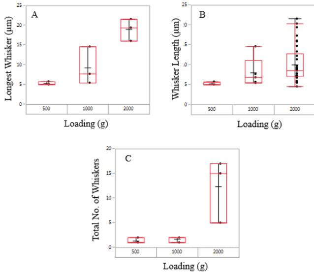
FIGURE 7. COMPARISON OF (A) THE LENGTH OF THE LONGEST WHISKERS. (B) THE WHISKER DISTRIBUTION AND (C) THE TOTAL NO. OF WHISKERS ON COATINGS TESTED WITH DIFFERENT LOADINGS (WHISKER TEST CONDITIONS: 1 µm FRESH TIN@10 ASD, 1mm DIA. BALL, 3 DAYS)
