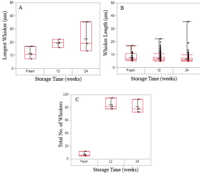
FIGURE 4 COMPARISON OF (A) THE LENGTH OF THE LONGEST WHISKERS, (B) THE WHISKER DISTRIBUTION AND (C) THE TOTAL NO. OF WHISKERS ON THE SAME SAMPLE STORED AT ROOM TEMPERATURE FOR DIFFERENT TIME (WHISKER TEST CONDITIONS: 1 µm @ 10 ASD, 2000 g LOADING, 1mm DIA. BALL, 3 DAYS)
