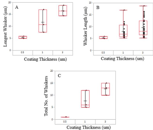
FIGURE 6. COMPARISON OF (A) THE LENGTH OF THE LONGEST WHISKERS, (B) THE WHISKER DISTRIBUTION AND (C) THE TOTAL NO. OF WHISKERS ON THE COATINGS WITH DIFFERENT THICKNESS (WHISKER TEST CONDITIONS: FRESH TIN@10 ASD, 2000 g LOADING, 1 mm DIA. BALL, 3 DAYS)
