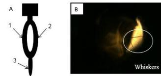
FIGURE 3. (A) ILLUSTRATION OF THE POSITION ON THE PINS FOR THICKNESS MEASUREMENT AND (B) TIN WHISKERS INSIDE THE HOLE WITH ENIG FINISH
