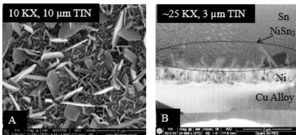
FIGURE 5. (A) TOP VIEW AND (B) CROSS-SECTION VIEW OF THE IMC FORMED BETWEEN NICKEL AND TIN STORED AT ROOM TEMPERATURE FOR 7 MONTHS
