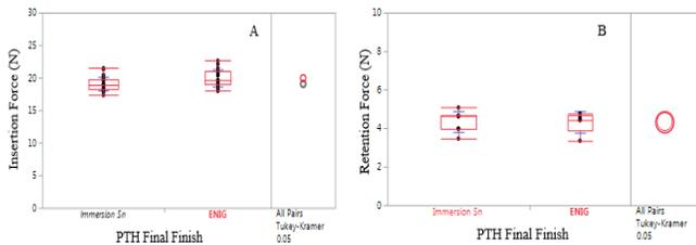
FIGURE 10. COMPARISON OF (A) INSERTION FORCE AND (B) RETENTION FORCE ON PTHS WITH IMMERSION TIN AND ENIG FINAL FINISHES
