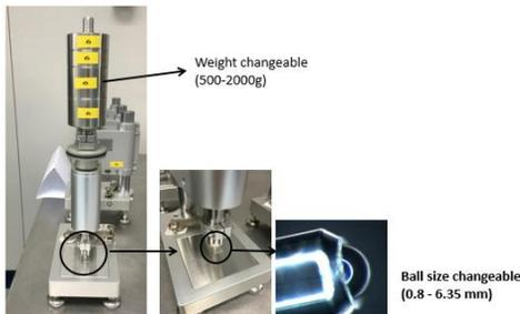
FIGURE 2. PHOTOS OF THE NEWLY DESIGNED WHISKER TEST SETUP
