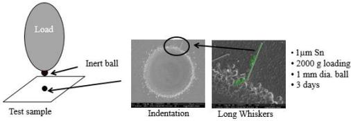
FIGURE 1. SCHEMATIC DIAGRAM OF THE INDENTATION METHOD FOR EXTERNAL PRESSURE INDUCED WHISKER GROWTH
