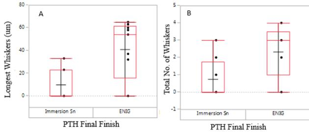
FIGURE 11. COMPARISON OF (A) THE LENGTH OF THE LONGEST WHISKERS AND (B) THE TOTAL NO. OF WHISKERS ON PTHS WITH IMMERSION TIN AND ENIG FINAL FINISHES
