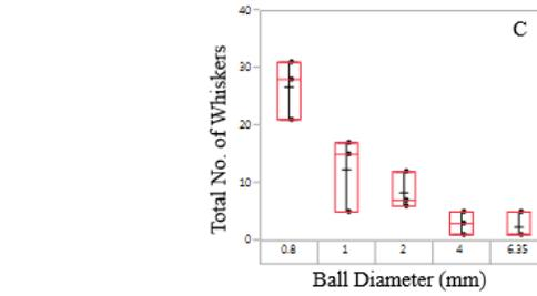
FIGURE 8. COMPARISON OF (A) THE LENGTH OF THE LONGEST WHISKERS, (B) THE WHISKER DISTRIBUTION AND (C) THE TOTAL NO. OF WHISKERS ON COATINGS TESTED WITH DIFFERENT BALL SIZE (WHISKER TEST CONDITIONS: 1 µm FRESH TIN@10 ASD, 2000 g LOADING, 3 DAYS)
