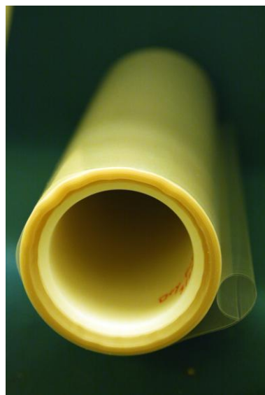
Figure 6. BCB laminate dielectric on plastic core
