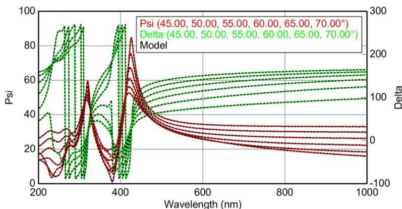
Figure 1: Variable angle spectroscopic ellipsometry data taken on a vapor-deposited 50 nm thick film of HTL A. The experimentally obtained psi (red) and delta (green) data are shown along with the anisotropic GenOsc modeling results (dashed, black line). The incident angles, relative to the surface normal, are given in the figure legend.
