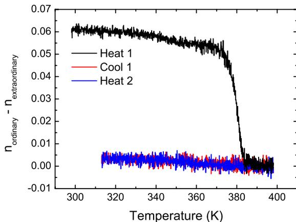
Figure 6: Difference between the ordinary and extraordinary indices of refraction as a function of temperature for a nominally 75 nm thick NPD film. A heat-cool-heat thermal profile performed at a rate of  $\pm 2$  °C/min was used, and the results are shown as the black, red and blue lines, respectively.
