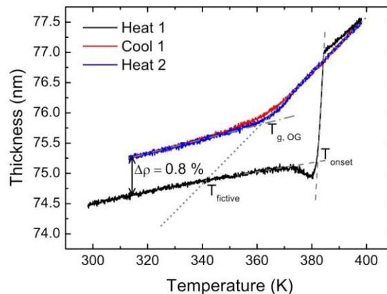
Figure 5: Thickness vs. temperature data for a nominally 75 nm thick NPD film vapor-deposited onto a silicon wafer with native oxide. A heat-cool-heat thermal profile performed at a rate of  $\pm 2$  °C/min was used and is shown as the black, red and blue lines, respectively.
