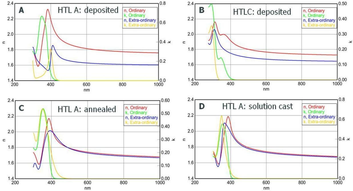
Figure 2: Index of refraction,  $n$ , and extinction coefficient data,  $k$ , obtained from model fits to VASE data for two different HTL materials. HTL A is also shown as a function of processing condition. The ordinary and extra-ordinary indices of refraction are shown as red and blue lines, respectively. Ordinary and extra-ordinary extinction coefficients are shown as the green and yellow lines, respectively.
