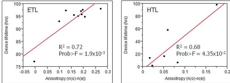
Figure 4: Correlation of device lifetime with anisotropy  $n(o)-n(e)$  measured at 632.8 nm) for the HTL and ETL materials studied in this proceeding. The correlation coefficient ( $R^2$ ) and the results of the F-test for an analysis of variance (ANOVA) are given for each material type.
