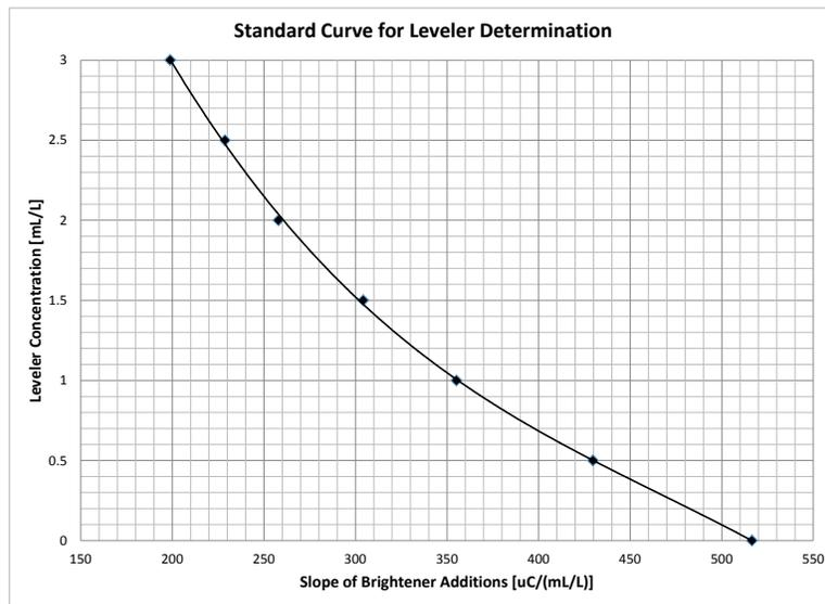
**Figure 8 – Standard curve for leveler determination.**
