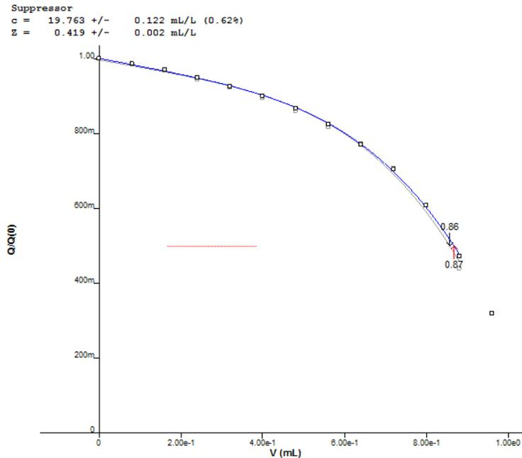
**Figure 5 – Suppressor analysis showing the standard curve and the sample curve overlaid (analyzed as 19.763mL/L suppressor). The red line denotes the arbitrary endpoint of 0.5x the initial mC reading of the blank (initial mC readings are normalized to 1.00).**
