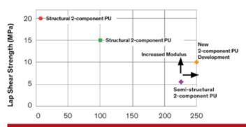
Figure 6 - Strength and elongation properties of structural PU adhesives.
