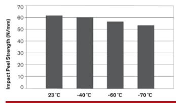
Figure 3b - Impact peel strength for various test temperatures.
