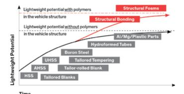
Figure 1 - New weight-reduction potential with structural adhesives and structural foams.
