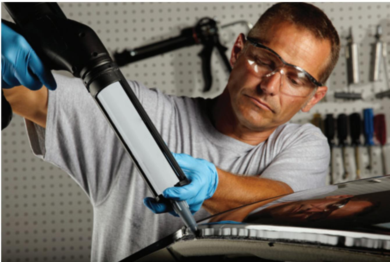
For all glass bonding installations, using cleaner-primer-adhesive systems from the same manufacturer is recommended for best results.
