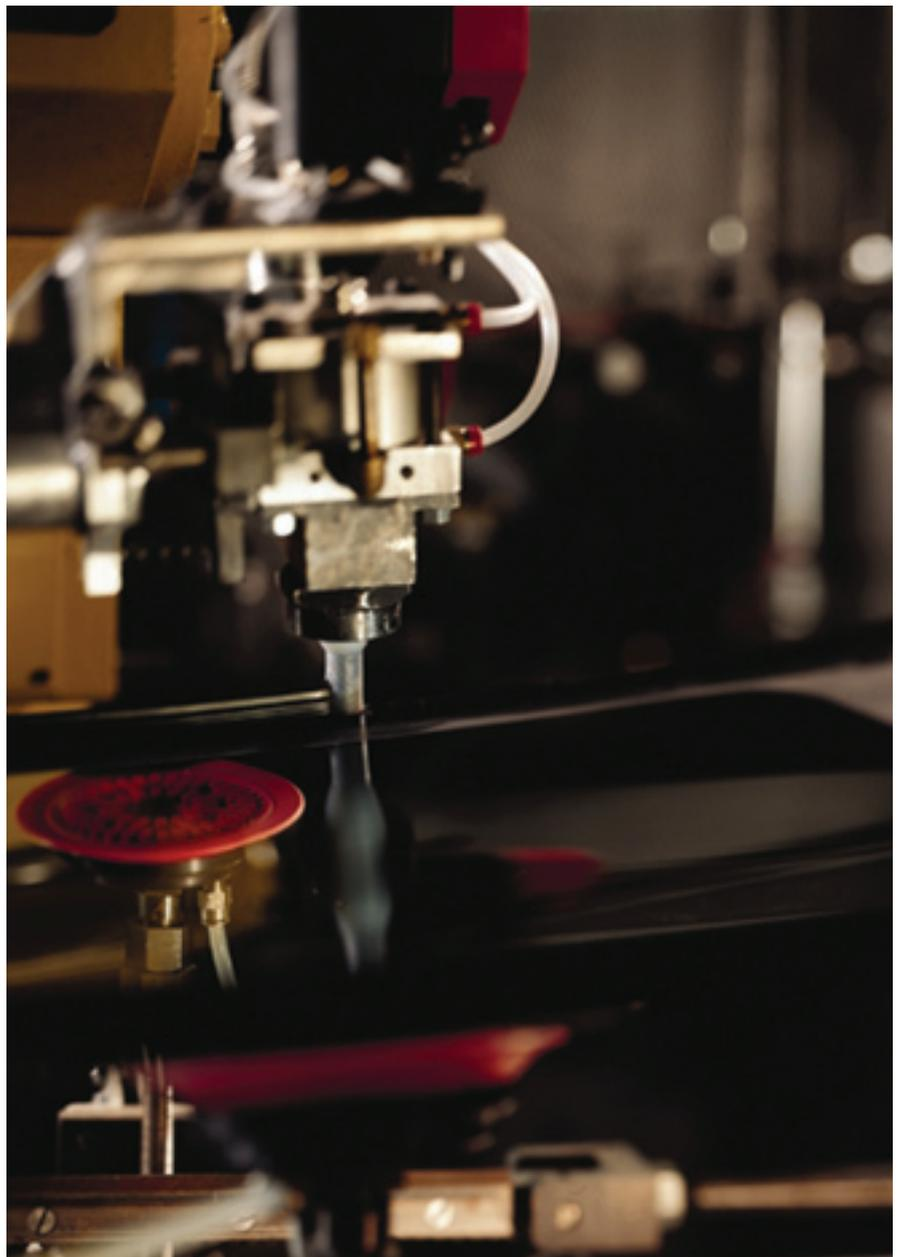
Robotic application of a glass bonding adhesive onto a windshield.
