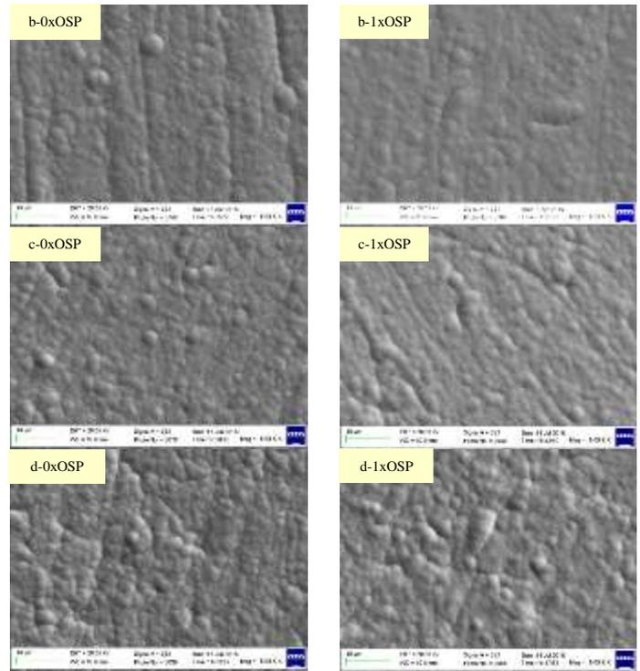
Figure 3: SEM images of EN surface for as-plated (0 x OSP) and after OSP simulation (1 x OSP; copper etch 0.75µm) of ENIG after gold stripping; (a) 0 MTO (b) 2 MTO (c) 6 MTO and (d) 12 MTO.
