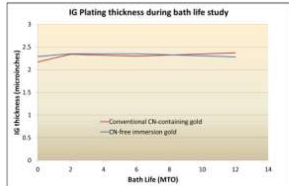
Figure 1: Comparison of IG plating thickness for the CN-free immersion gold bath (45°C, 11 min) and Conventional CN-containing gold bath (84°C, 8 min) as a function of bath life.
