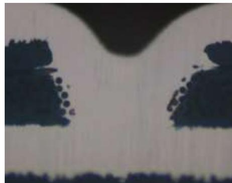
FIGURE 3. OPTICAL MICROSCOPE IMAGE OF MICROVIA CROSS-SECTION AFTER LLTS
