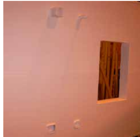
Figure 2: Penetrated Wall Configuration for ASTM E2357 Testing of DuPont™ Tyvek® Fluid Applied Assemblies
