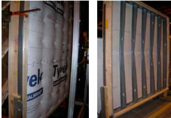
Figure 6. Phase II: Structural High Pressure Performance Testing
