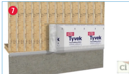
7. Install DuPont™ Tyvek® ThermaWrap™ R5.0, working from the bottom up and right-to-left.
