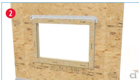
2. Bump-out frame around all window and door openings and penetrations larger than 1".
