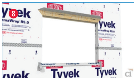
8. Cut and prepare window/door openings.
