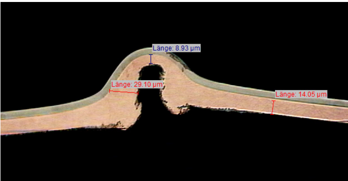
Poor copper throwing power
