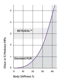
High modulus adhesives are stiffer than "standard modulus" adhesives, making the car body more rigid, and reducing noise, squeaks and rattles.
