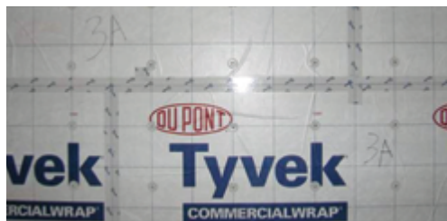
Figure 2: Opaque Wall Configuration for ASTM E2357 Testing of DuPont™ Tyvek® Commercial Building Wrap Assemblies
