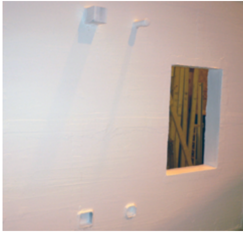
Figure 4: Penetrated Wall Configuration for ASTM E2357 Testing of DuPont™ Tyvek® Fluid Applied Assemblies
