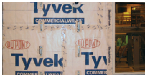
Figure 3: Penetrated Wall Configuration for ASTM E2357 Testing of DuPont™ Tyvek® Commercial Building Wrap Assemblies
