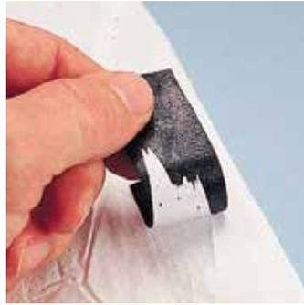
Microporous films rely on thin film for barrier.
