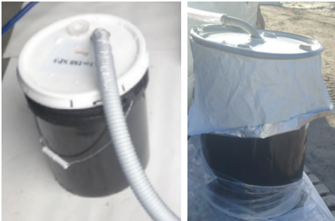
Siphon hose inserted through integrated pouring spouts of the 5-gallon bucket (left) and 55-gallon drum (right) with vacuum-sealed bag folded over drum walls and dip tube connected to siphon hose”
