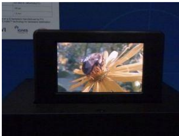
DuPont 4.3-inch printed OLED prototype
