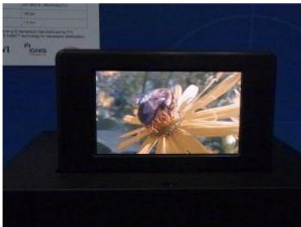
**DuPont 4.3-inch printed OLED prototype**
