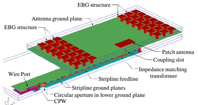
Fig. 1. Features of the 60 GHz LTCC patch antenna.
