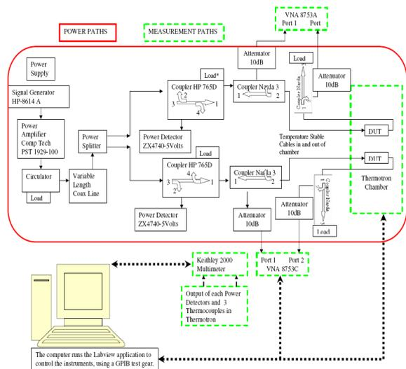
Figure 3: Layout of the RF test setup
