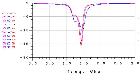
Figure 1 B: Measured Transmission spectrum of the test filter.
