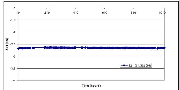
Figure 8: Insertion loss of the filter at 1.332 GHz over time.
