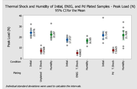
Fig. 3 Thermal shock & humidity adhesion peak load (N).
