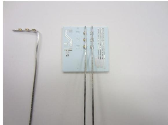
Fig. 5 Loss of adhesion wire during testing.
