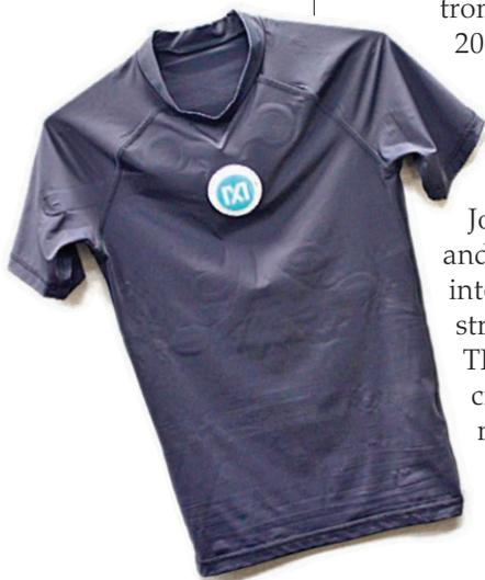
Thin thermoplastic polyurethane films printed with DuPont Microcircuit Materials' stretchable conductive inks are bonded strategically to the inside of a fitness shirt (bottom left) to provide biometric function.
