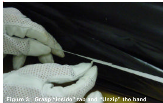
Figure 3: Grasp "inside" tab and "Unzip" the band
