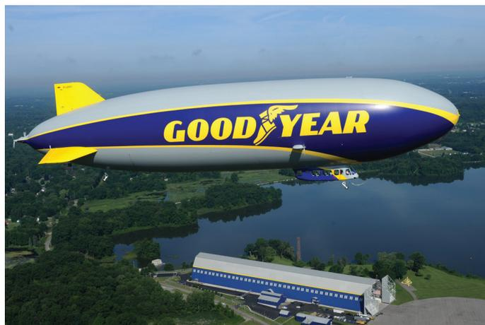
The body, or envelope, comprising the airship's largest component, holds the helium that makes the blimp lighter than air. The new blimp has a volume of 297,527 cubic feet, and is 246 feet long – 50 feet longer than the previous blimp. The outer covering, or envelope, surrounds a semi-rigid internal structure, which is a departure from the unsupported envelopes used in previous Goodyear blimps.
