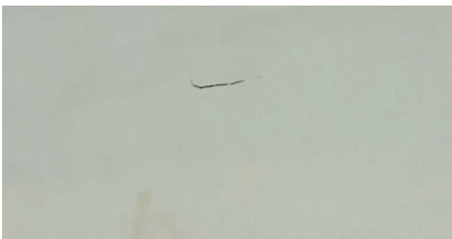
Figure 10. This pouch made with 85g Reinforced Paper / 11.5g Allover Coating had a confirmed puncture.
