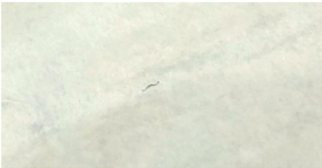
**Figure 9.** This pouch made with 60g Paper / 11g Grid Lacquer had a confirmed puncture.
