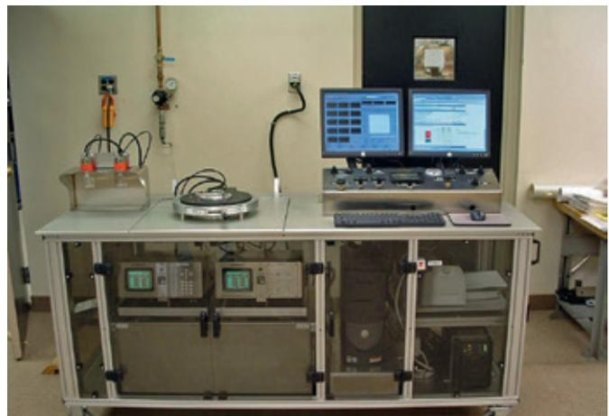
**Figure 4. Microbial barrier test system (ASTM F2638).**
