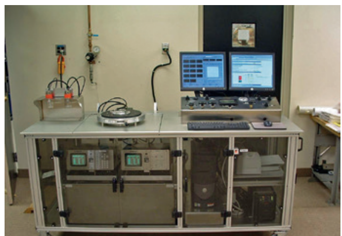
Figure 4. Microbial barrier test system (ASTM F2638).
