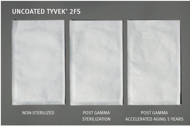
Figure 11. Medical-grade papers show yellowing after being sterilized by Gamma radiation. None of the pouches made with Tyvek® 1073B or Tyvek® 2FS™ showed any discoloration.
