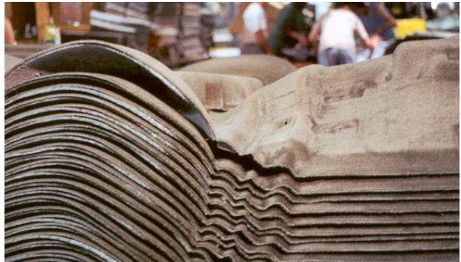
Magee Rieter Automotive supplies carpet and other interior components made with DuPont™ Keldax® resins for such GM models as the Chevrolet Trailblazer, GMC Envoy, Oldsmobile Bravada and the Cadillac STS (shown). Components made from Keldax® retain their shape for easy installation and a precise fit.
