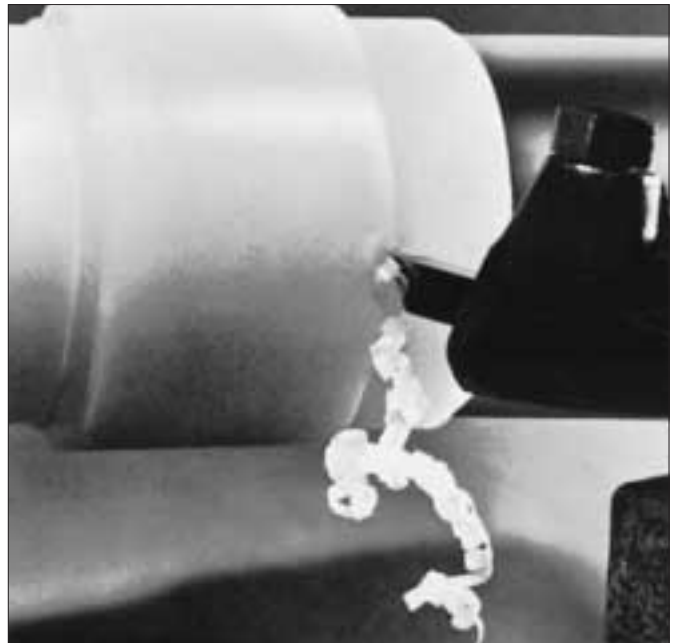
Fig. 11.04 Turning Machining conditions: Lathe speed, 980 rpm; cutting speed 185 m/min; feed 0,15 mm; depth of cut, 2,5 mm; No coolant. Material – ZYTEL® 101 – 60 mm diameter.
