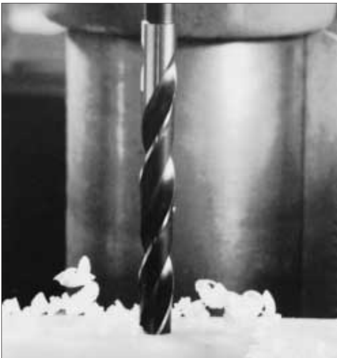
Fig. 11.03 Drilling Machining conditions: Drill size, 10 mm; Speed 1000 rpm; No coolant. Material – ZYTEL® 101 – 35 mm thick.
