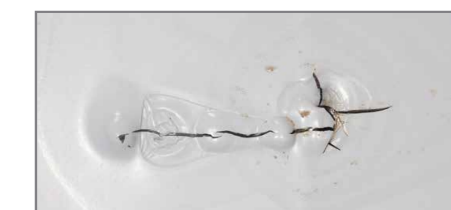
High intensity hot spots in PVDF-based backsheets
