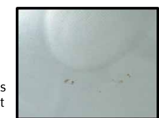
Delamination of PVDF-based backsheet on 134°C hot spot.
