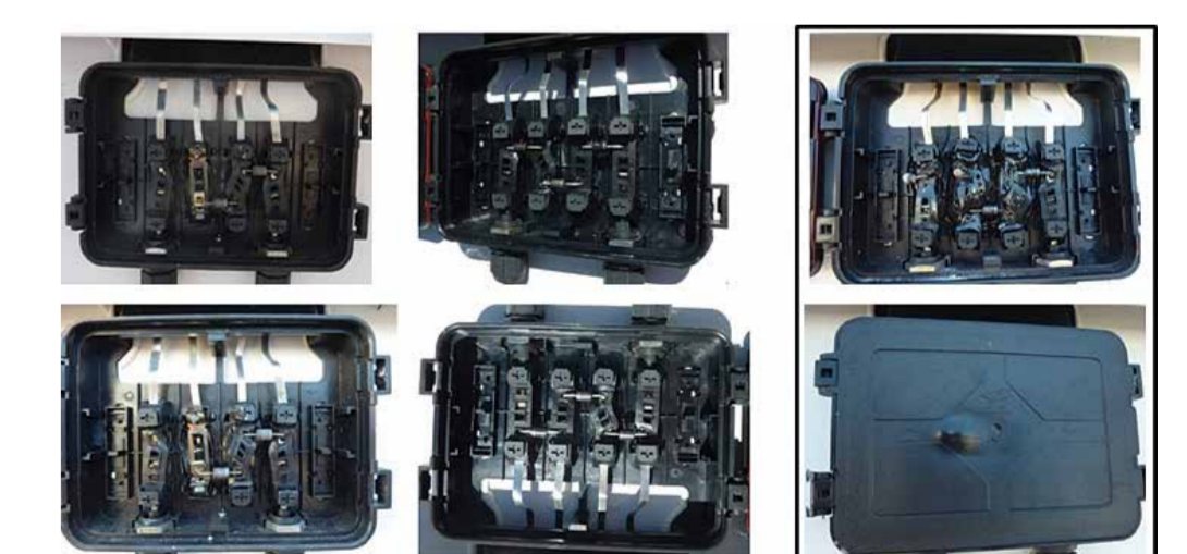
Example of bypass diode overheating and subsequent junction box melting.
