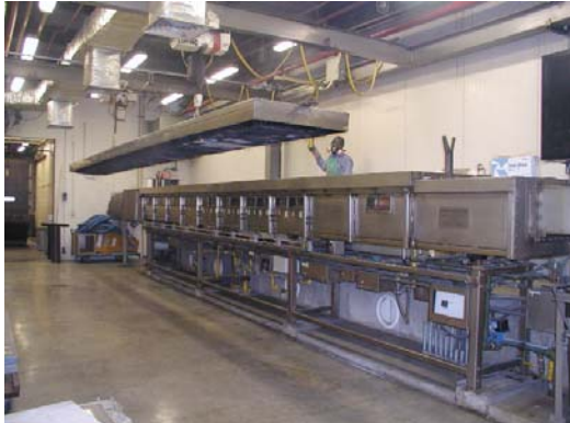
Figure I: Exterior view of the Steiner Tunnel apparatus: Underwriters Laboratories Inc., Northbrook Division, Northbrook, Illinois. Tunnel or chamber lid is removed completely for insertion of test material.
