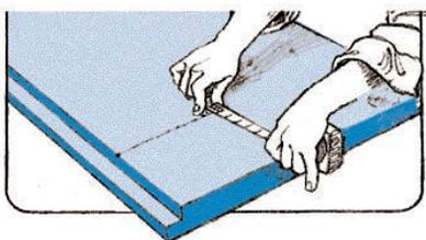
2. To cut, hold utility knife low against the board and make a deep impression. There is no need to cut all the way through.
