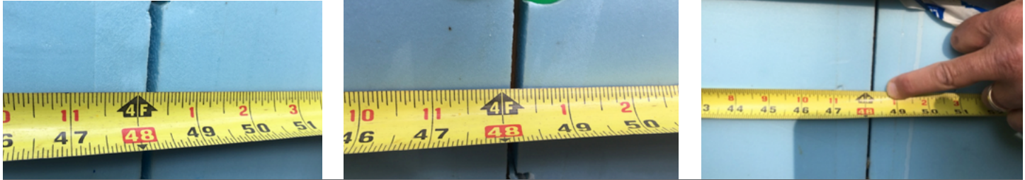
Photo 8a, b, c; width dimension measurement of three boards with intact factory edges
