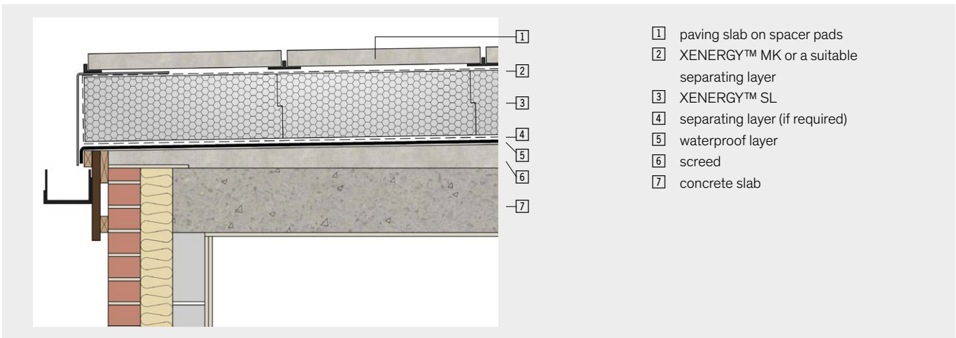
Figure 6 Ballasted inverted roof - detail at eaves
