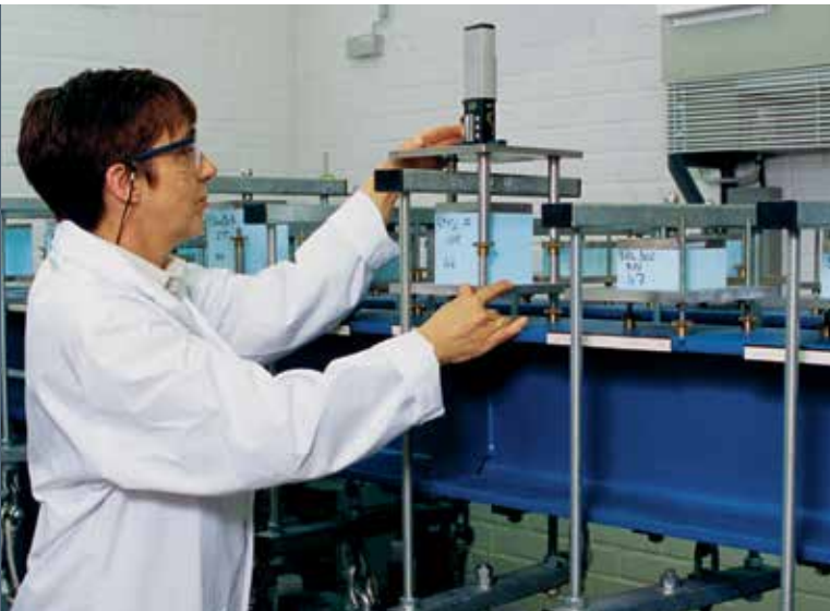
Fig. 16: Testing creep rupture behaviour under a compressive load in accordance with DIN EN 1606
