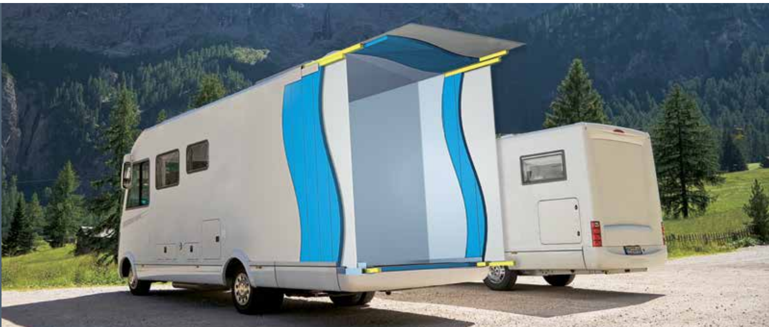
Fig. 01: Motorhome cross-section (simplified illustration to clearly explain the use of STYROFOAM™)
