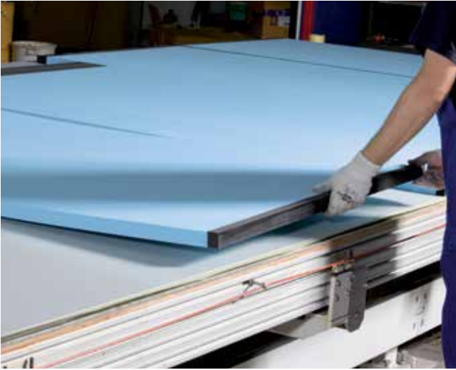
Fig. 10: Aligning STYROFOAM™ panels
