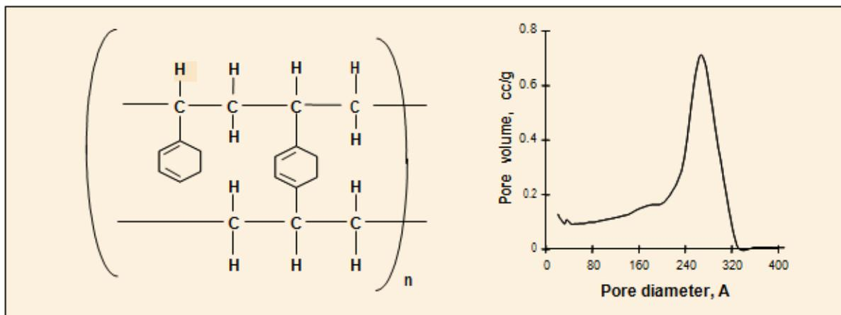
Figure 2 : Pore distribution of AMBERLITE XAD16N polymeric adsorbent
