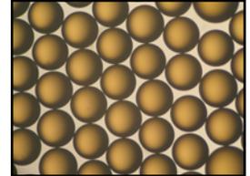
AMBERLITE™ IRN97 H is a higher capacity, 10% DVB cation resin used to remove cations for purification and pH control in primary water treatment. It contains a minimum of 99% of its exchange sites in the hydrogen form. The uniform particle size and the absence of fine resin beads result in a lower pressure drop compared to conventional resins.
